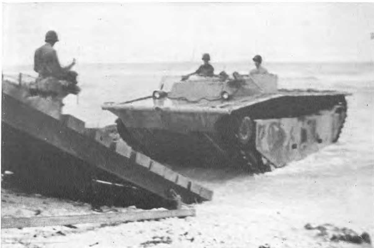
READY FOR BUSINESS the special portable LVT ramp supported vehicles up to and including 35-ton tanks.
