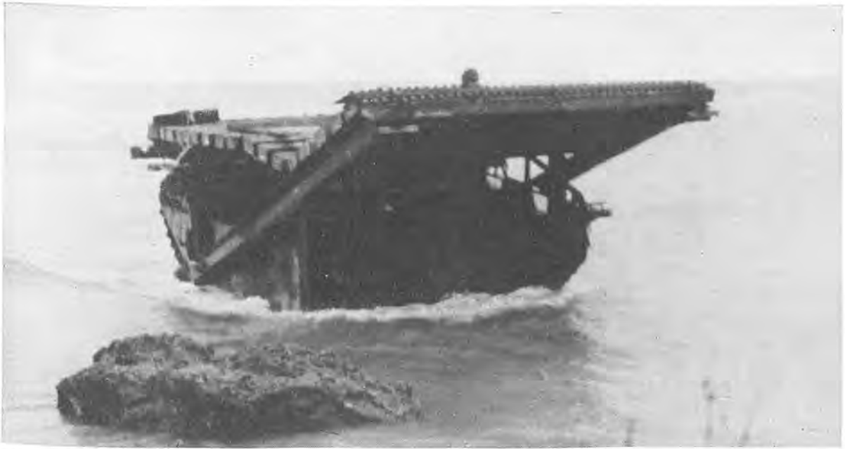
SPECIAL PORTABLE LVT RAMP was designed to provide access over the coral ledges flanking the landing beaches. After placing the ramp's forward end against the top of the ledge and securing the after end at the base, the LVT backed away, allowing the ramp timbers to fall into position on steel I-beams.
