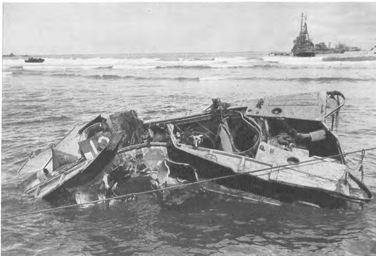
DEMOLISHED LVT , one of three that ran over and detonated Japanese mines on White 2. One hundred horned mines, many of them unarmed, were eventually removed from White 2 and surrounding area.
