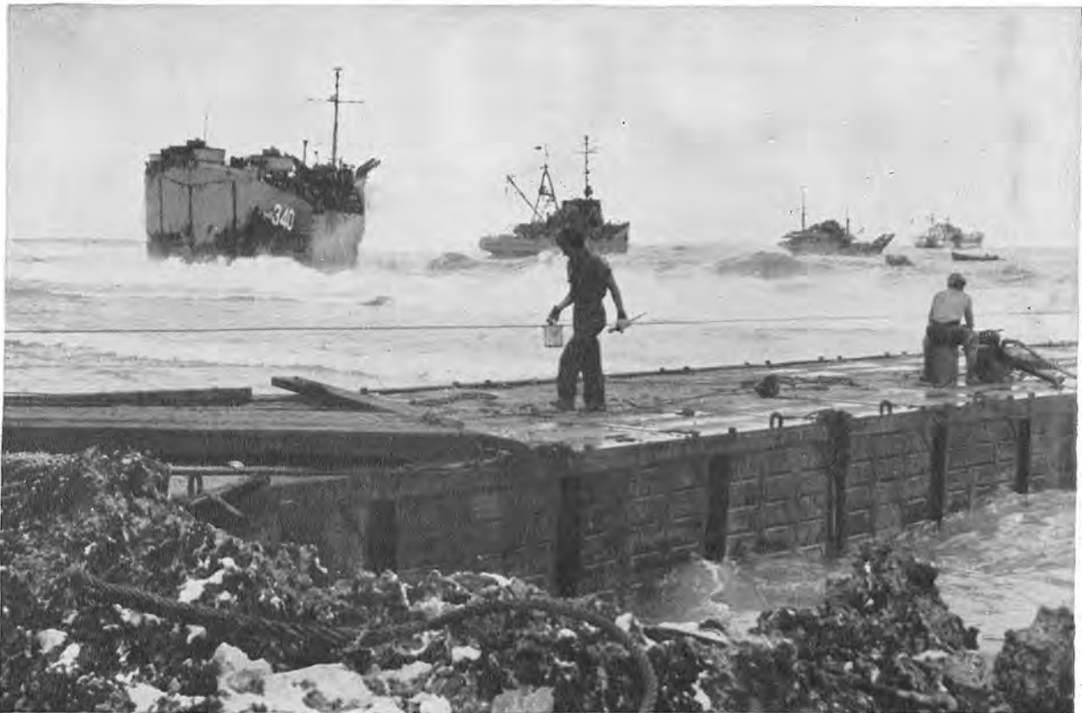
GROUNDING LST off Beach White 2. After unloading 24 trucks on the pontoon causeway and taking aboard a load of 200-odd casualties, the ship attempted to retract. Then, during a sudden squall, she broached on the reef. Casualties aboard her were transferred the next day to another ship.
