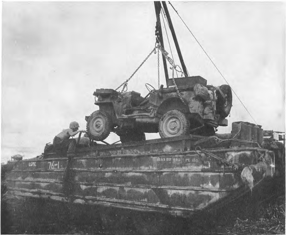
DUKW UNLOADS JEEP by means of "A" frame, which lifts vehicle from the truck and places it on the ground. The 140 DUKW's available to the landing force fulfilled an urgent need at Tinian, especially after 1800, Jig-plus 4, when rough weather precluded all unloading by means other than DUKW's.
