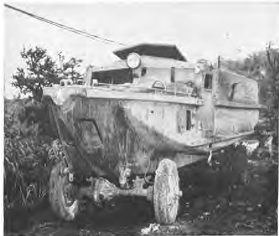
JAPANESE AMPHIBIAN TRUCK , one of several captured at Tinian. It operated as a conventional 4x4 truck on land and could function afloat by disengaging the front-wheel drive and engaging a propeller on the vehicle's stern.
