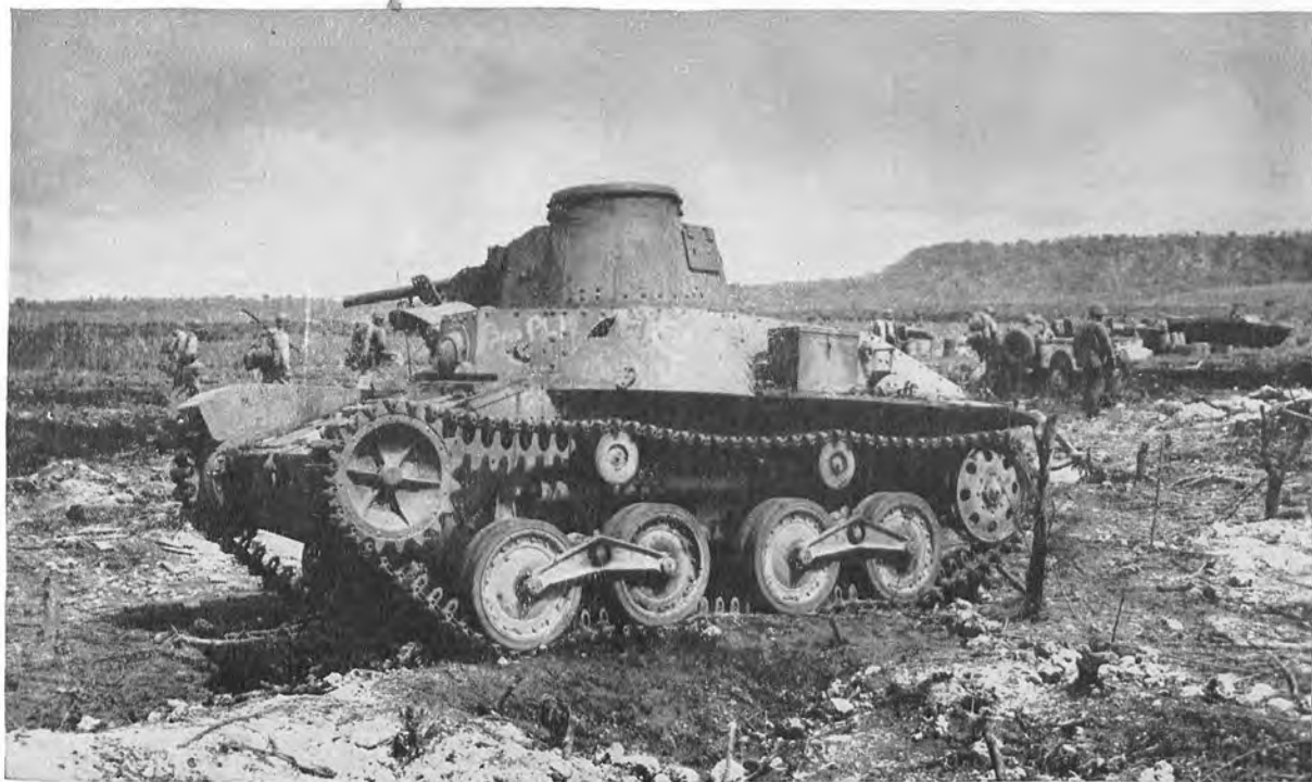
JAPANESE TANK , one of five knocked out during the first night's battle. All Japanese tanks on Tinian were light models mounting 37mm guns and 7.7cm machine guns.
