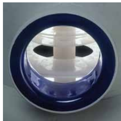
Glass-lined column shell with PVDF internals
