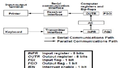
The 1 bit FGI is a control flip flop that sets to 1 when new data is available in input device and cleared to m0 (by processor) when computer receives it (needed to synchronize time difference between processor and input device).
