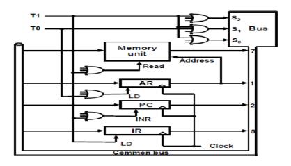
A portion of bus system that shows hardware implementation of micro-operations taking place during T0 and T1
