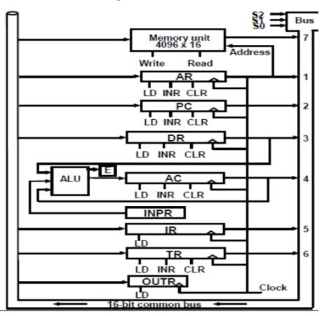
Three control lines, S2, S1, and S0 control which register the bus selects as its input and so the selected register will issue its output to the bus.
