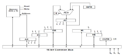
Any and only one source of those register can be selected to apply its content to the bus and during the same clock cycle the bus content could be directed to one or many destinations of registers or memory unit. For example we can do the next micro-operation:
