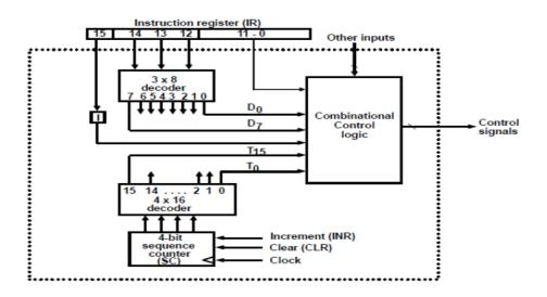
Sequence counter is used to synchronize action with those 16 different time intervals.
