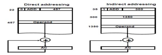
The previous figure shows an example of addressing mode. In location 22 there is an ADD instruction that adds the AC with operand in location 457 as an indication for direct addressing mode as I=0.
