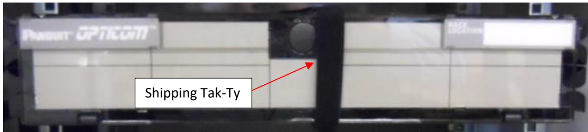
2. Figure 5: Shipping tape to be removed from FRME1U.
