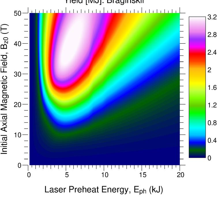
Figure 4. Parameter scan across  $E_{ph}$  and  $B_{z0}$  for the fusion yield,
