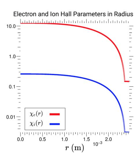
Figure 2. Electron and ion Hall (2) after laser preheat ends, when  $T_q(r=0) \approx 1$  keV.
