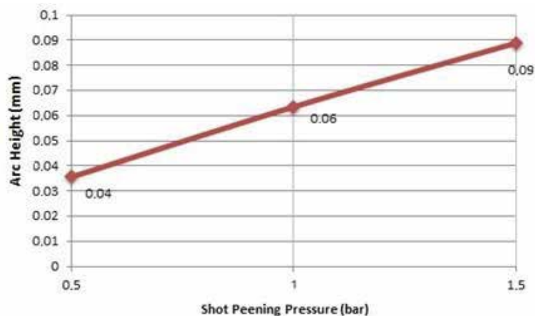
Figure 3. Correlation between the arc height and shot peening pressure.
