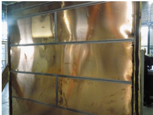
Figure 15.6.1: Horizontal copper flat lock panel with taped joints to isolate joinery elements for ASTM E283 air flow testing.
