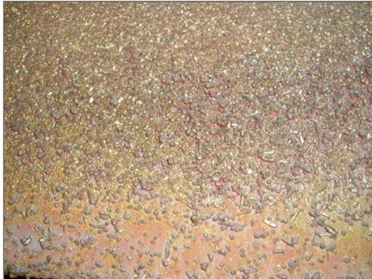
Figure 3.1A. As natural a look as you can get: unfinished copper cathode, 99.9% pure. Typically shipped as melting stock to mills or foundries, cathodes may also be cast into wire rod, billets, cakes or ingots and alloyed with other metals.
