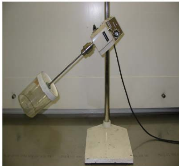
Fig. 22. Top secured overcoater used in early development stages of AGR-1 test article development [36].
