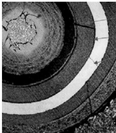
Fig. 76. Irradiated particle with through cracks in all of its coating layers (iPyC, SiC, oPyC, and an outer protective layer).
