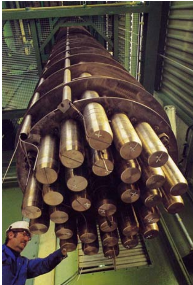
Fig. 89. Reformer tube test bundle for the generation of synthesis gas under simulated nuclear conditions in the EVA-II facility at the Research Center Juelich.
