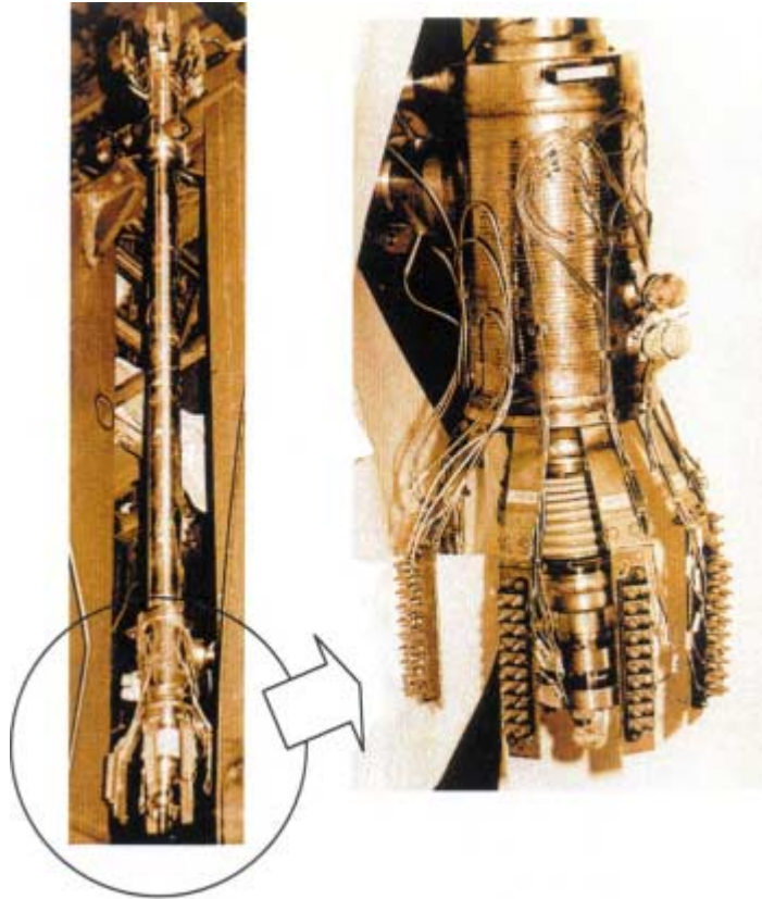
FIG. 7. Tests of full-scale heat exchange element at helium test facility.
