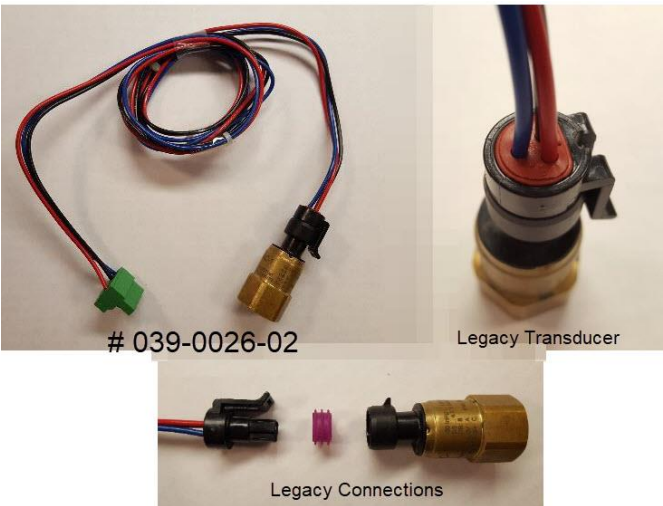
Figure 16 – Part # 039-0026-02 Legacy pressure transducer and cables.
