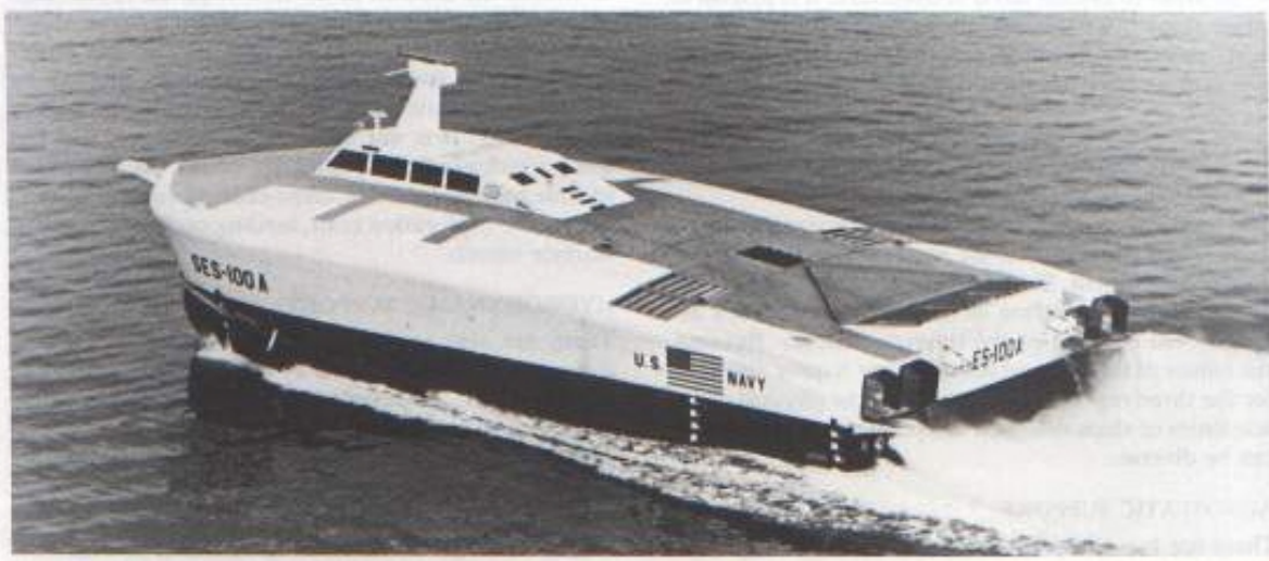
Figure 1-2. Another type of surface effect ship, a captured-air-bubble vehicle (CAB), is supported on a cushion of air that is screened at the sides by the rigid side structure of the vessel.
