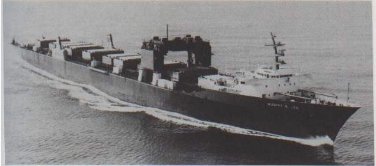
Fig. 3 SS ROBERT E. LEE—LASH barge carrying ship built in 1974 by Avondale Shipyards, Inc. for Waterman Steamship Corporation; Molded dimensions 272.3 m (893.3 ft) by 30.48 m (100 ft) by 18.3 m (60 ft)
