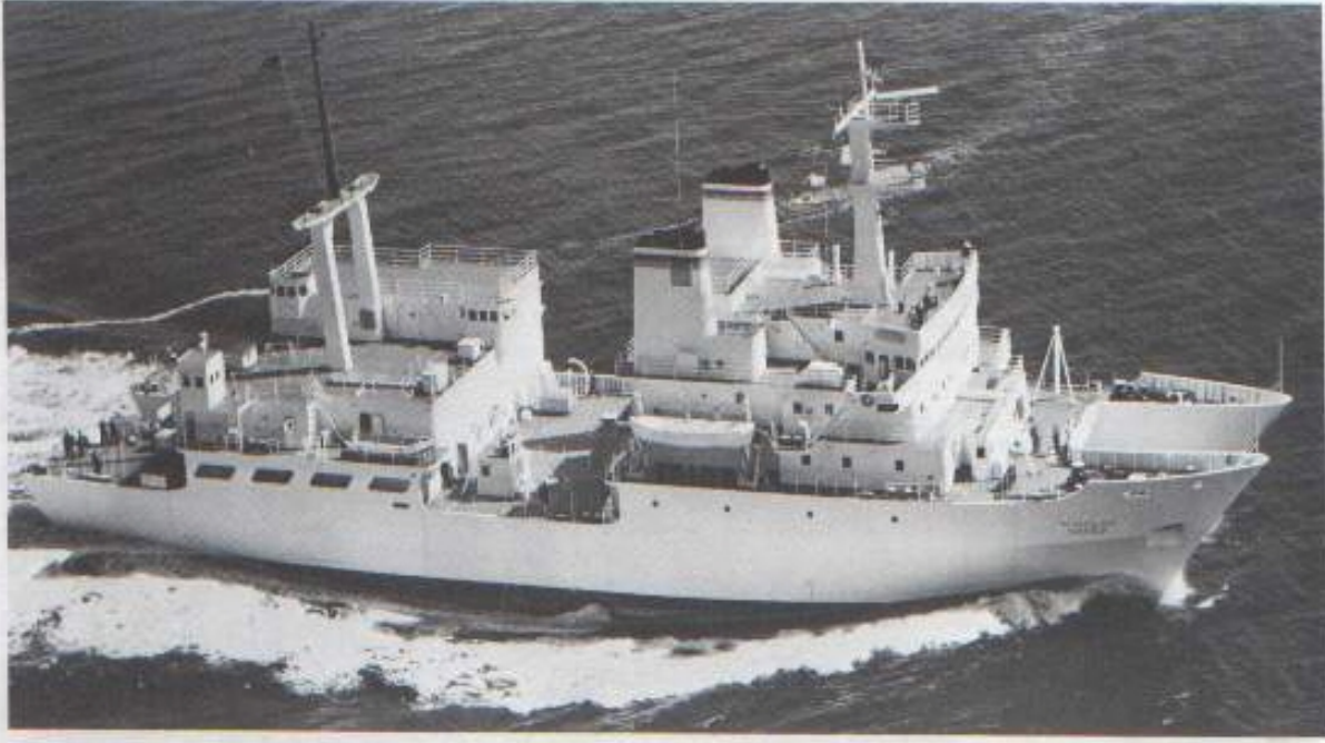
Figure 1-11. The oceanographic research vessel USNS Hayes , one of the best examples of a multi-hull vessel, generally a costly, controversial type
