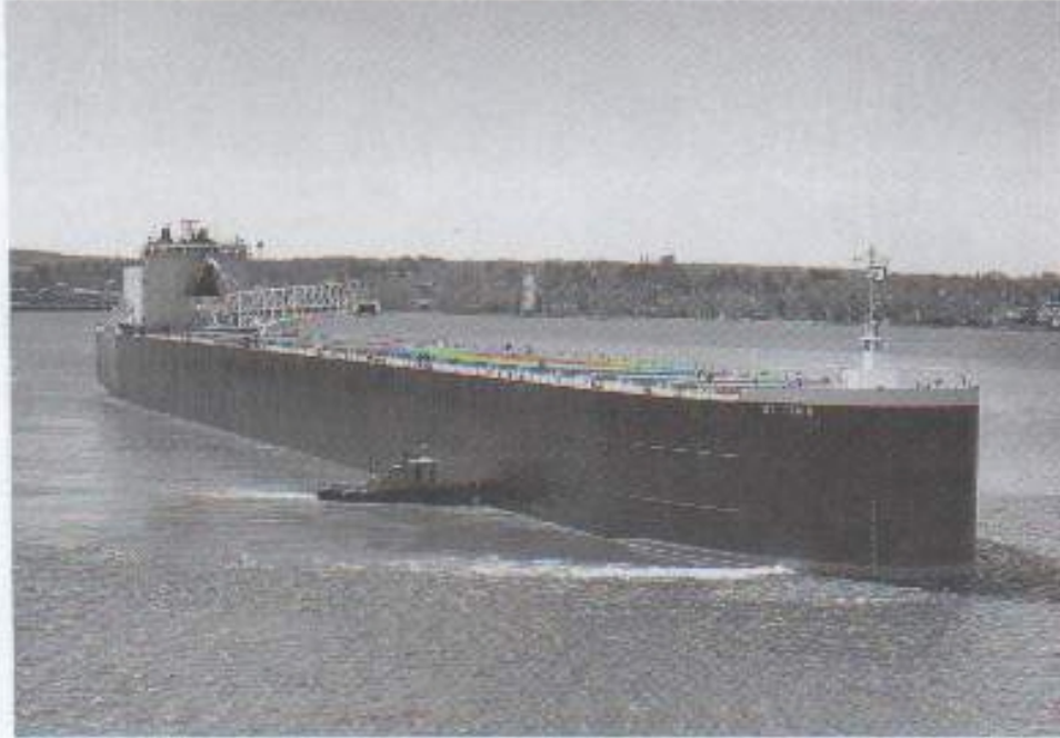
Fig. 2.9 Two kinds of bulk carriers. Upper: Tanker Esso Le Havre , of 381 000 deadweight tons. This was the first vessel of such an extreme size to transit the Suez Canal (in 1981). Courtesy R.F. Klausner, Exxon Company, International. Lower: Self-unloading collier St. Clair , typical of Great Lakes bulk carriers. Photo by Har- mann Studios, Sturgeon Bay, Wisconsin.
