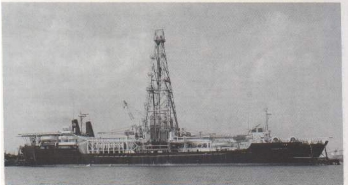
Fig. 10 GLOMAR PACIFIC—drilling ship built in 1977 by Livingston Shipbuilding Company, Inc. for Global Marine Inc.; Moulded dimensions 137 m (448.5 ft) by 21.9 m (372 ft) by 10.7 m (35 ft)
