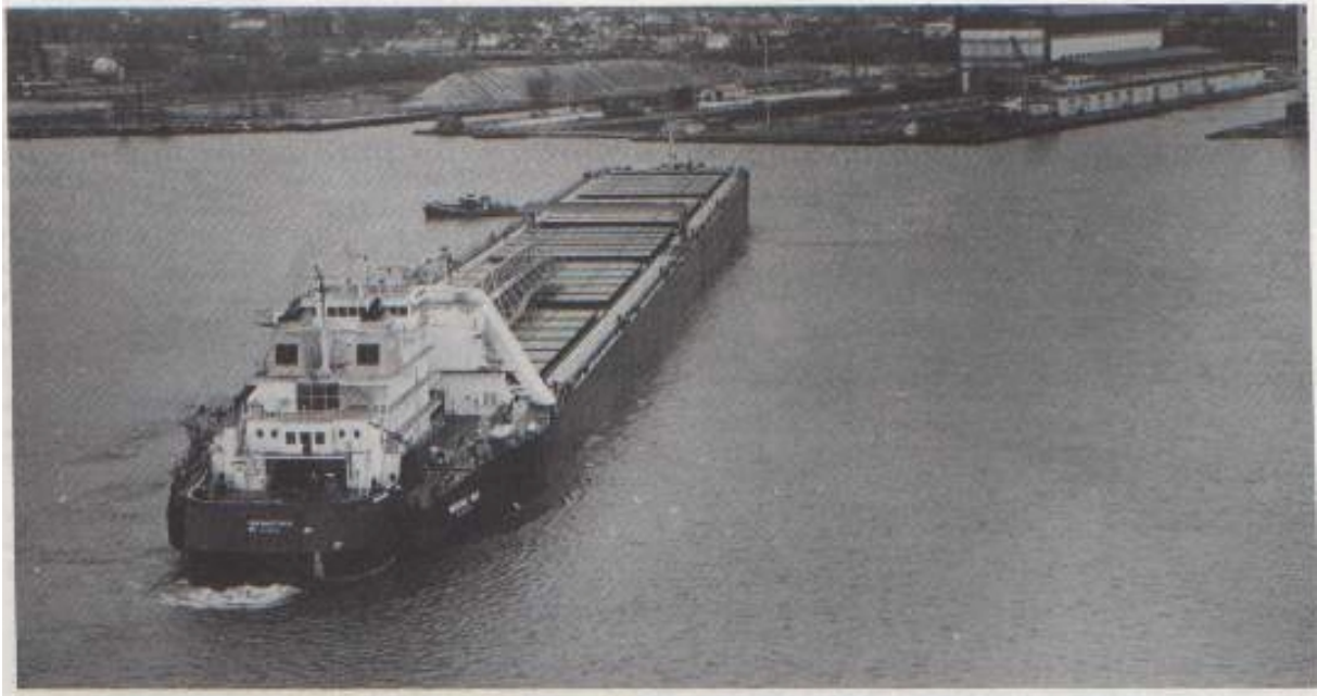
Fig. 8 ITB PRESQUE ISLE—integrated tug barge Great Lakes ore carrier built in 1973; tug built by Halter Marine Services; barge by Erie Marine, Inc. for Lilton Great Lakes Corporation; Moulded dimensions of integrated vessel 304.8 m (1,000 ft) by 31.9 m (104.6 ft) by 14.2 m (46.5 ft)
