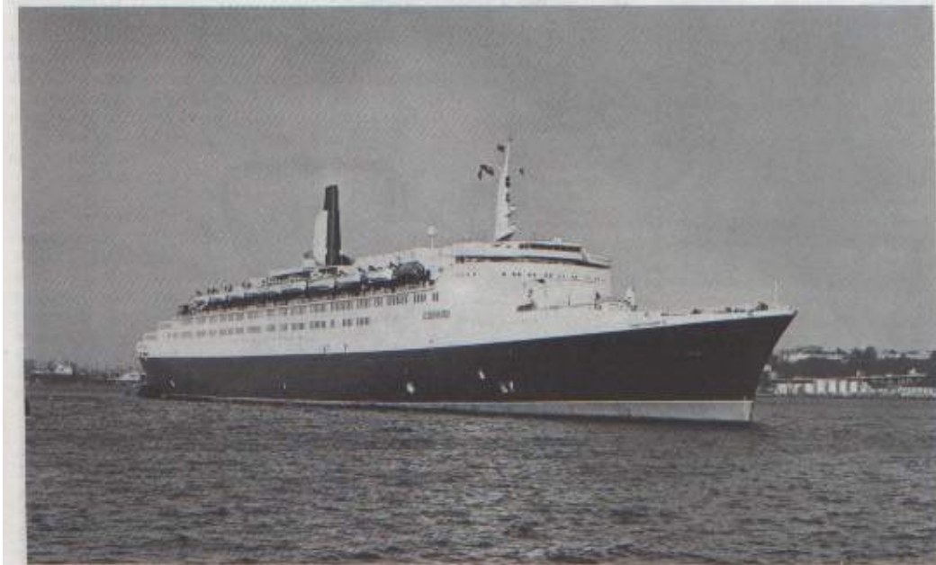
Fig. 9 SS QUEEN ELIZABETH 2 —passenger liner built in 1969 at John Brown Shipbuilding Company for Cunard Line Ltd.; Moulded dimensions 293.5 m (963 ft) by 32 m (105 ft) by 17.1 m (56 ft)
