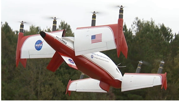
Figure 6.2: LA-8 flight test.
