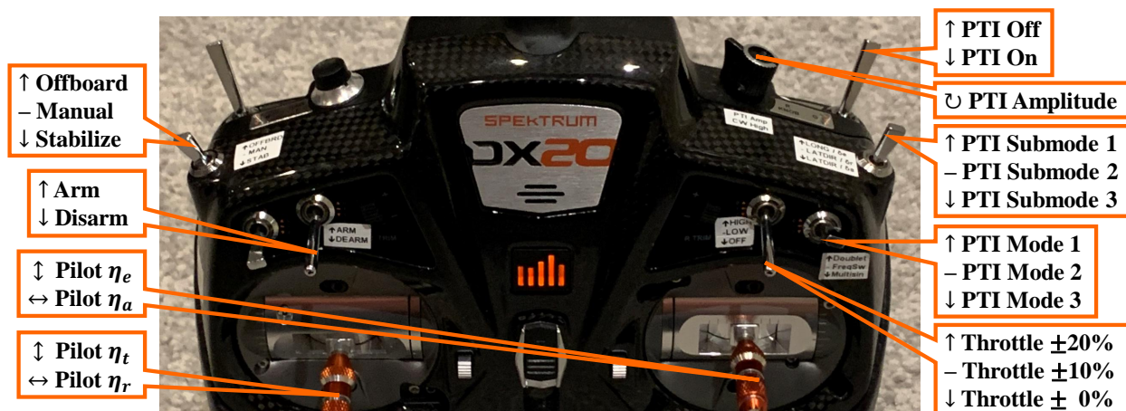
Figure 2.7: RC transmitter programmed for system identification flight testing.
