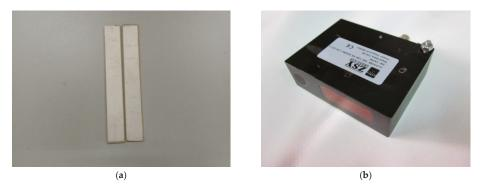
Figure 2. Scheme of experimental specimens and measuring instruments: (a) PbZrTiO<sub>3</sub>-5 (Generally abbreviated as PZT-5) piezoelectric ceramic specimens. (b) The non-contact laser displacement sensor.
