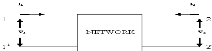
Fig(a) Two port network.
