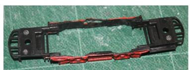
Then remove the entire lower saloon floor right up to the bulkheads and the body sides.
