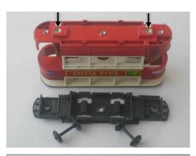
Remove the plastic base from the tram and drill off the heads of the next two rivets, shown by the arrows, holding the lower saloon doors and upper deck.
