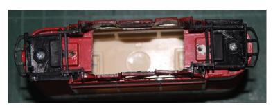
Attach the plastic under section using self-tapping screws.
