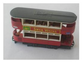
Read here how to motorise the HO scale (3.5 mm / foot) Matchbox Y-15 tram with a Halling Vario 23 mm wheelbase chassis and a Halling Old Timer tram base which is available as a Halling spare part. This, with platforms removed, will fit into the lower deck of the Matchbox tram and has four lugs which the power unit clips into.
