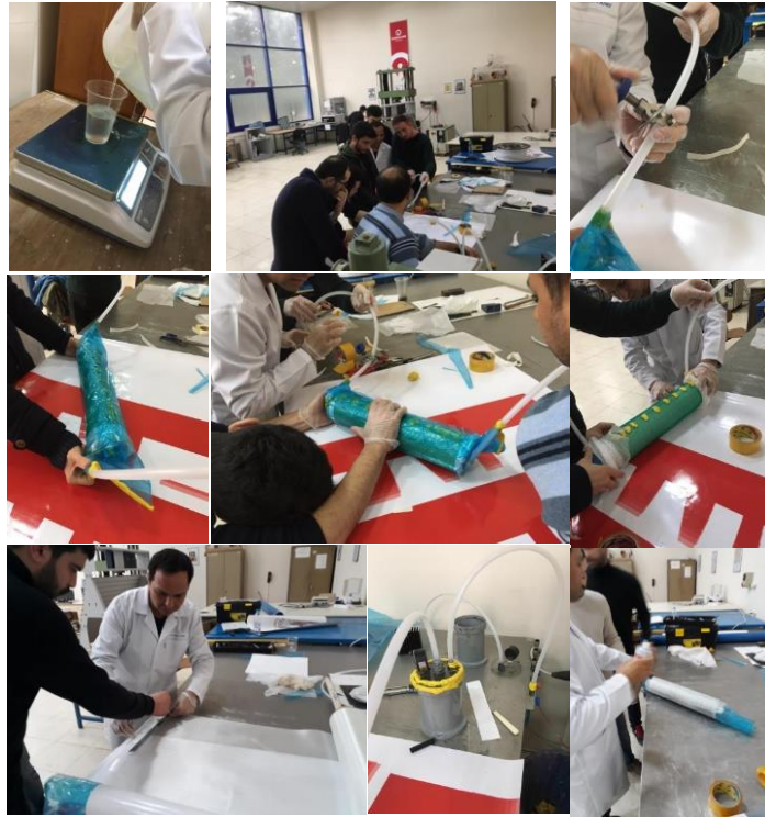
Figure 9. Manufacturing of Composite Body Pipe with Cylindrical Cross Section
