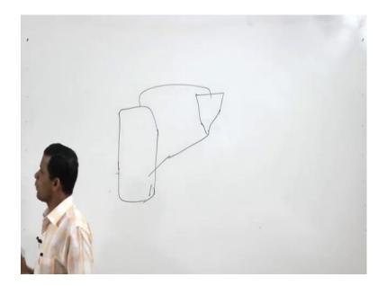
So, that will be separated in a cyclone and it will be recycled back, it will be recycled back to this. In this system we have some riser part like this as shown here and this is a close system operation is required for this, fluidized bed incinerator has some advantages as such it is suitable for high moisture fuel or low grade fuel, the typical operating temperature are lower than that of fixed bed higher combustion efficiency and more suitable for large scale operations.
