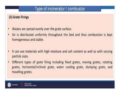
And different types of grates can be used like say it can be fixed grates, moving grates, rotating grates, horizontal or incline grate or water cooling grate, dumping grate and travelling grates. So, different types of grates can be used some of the important grates types are mentioned here that is reciprocating grate.
