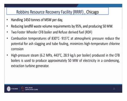
And combustion temperature is 830 to 915 degree centigrade, and high pressure steam is produced 6.2 mega Pascal and 443 degree centigrade, and that is produced in a circulatory fluidized bed boilers is used to produce approximately 50 megawatt of electricity up to this on this module.
