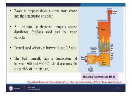
So, circulating fluidized bed use is more air velocity, and in that case part of solids has to be recycle back. So, this is bubbling fluidized bed. So, in case of bubbling fluidized bed we use intermediate velocity more than packed bed and lesser than circulating fluidized bed, and typical sand velocity for bubbling fluidized bed is 1 to 2.5 meter per second, 1 to 2.5 meter per second for bubbling fluidization. The bed normally had a temperature of
