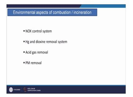
So, as per the flow sheet after boiler we have few gas clean up sections NOX, mercury removal dioxin removal, and acid removal and particulate metal removals are required and we will discuss this things in another chapter another module, we will now discuss some operational problems which is experienced during the operation of this incinerators; two important problems one is your slagging.
