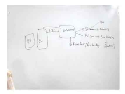
So, heat recovery is the second or third part of this, so pretreatment incineration and heat recovery. So, heat recovery is the third part of this and important part of this incineration process or flow sheets, hot gas when it comes in the boiler we may get steam we may get hot gas, gas turbine tow electricity steam to electricity, steam to any use or process heat to pre heating etcetera. So, we have number of options to use this hot gas.
