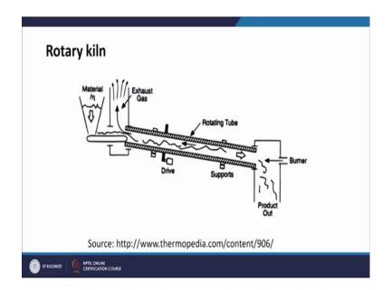
Now, this is the rotary kiln the operations we have already discussed and mechanism of waste burning and grates. We will see the grates provide sufficient time grates hold the material in the combustion chamber and helps for the contact of oxygen and waste
