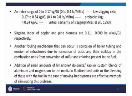
So, 0.17 to 0.34; 0.17 non slagging 0.17 to 0.34 slagging probably, but if it is greater than 0.34 slagging; the slagging index of popular and pine biomass are 0.11 and 0.009 kg
