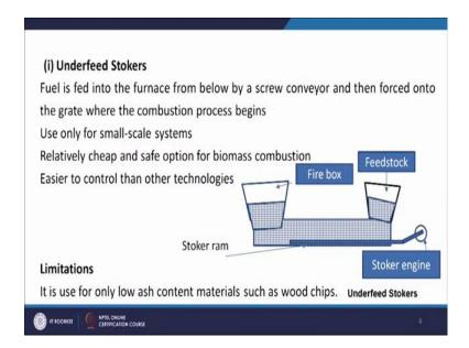
This is not very attractive and it has not very large applications it is limited applications and it is used for only low ash content materials such as wood chips, this is relatively cheap and safe option for biomass combustion and easier to control than other technologies.
